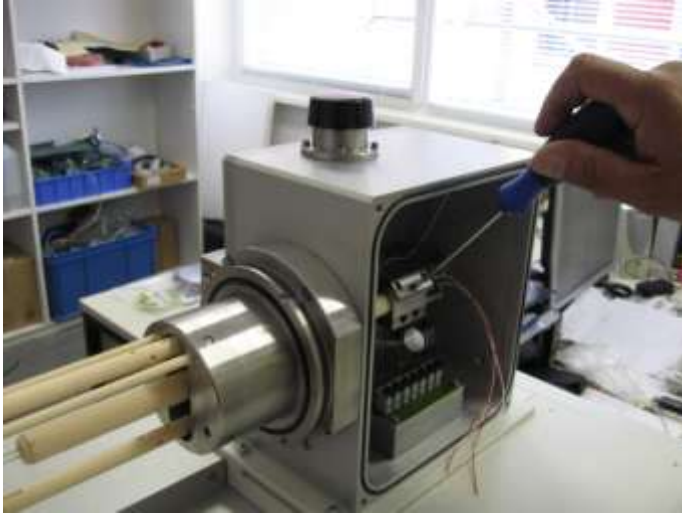
Pic 1: Open Locking Screw for removal
