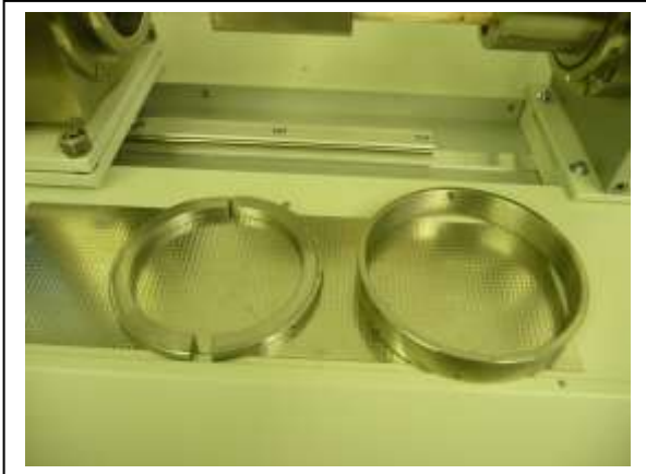
Remove the O-Ring at the chamber
