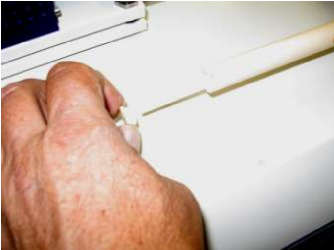
Pic 4: Pull out Al 2 O 3 Locking tube
