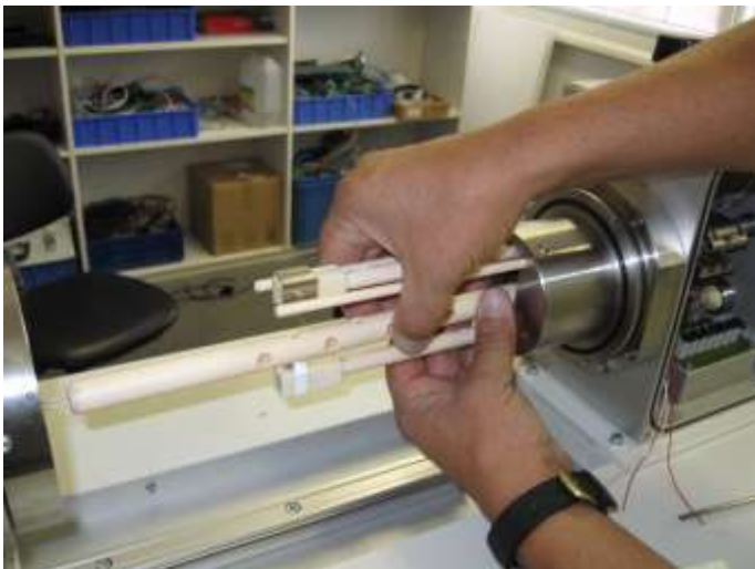
Pic 2: Pull out tube with 2 TC
