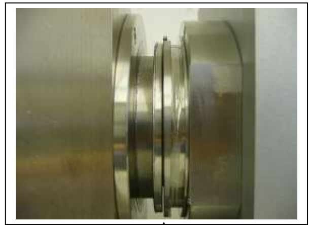
bad example gap at bottom
